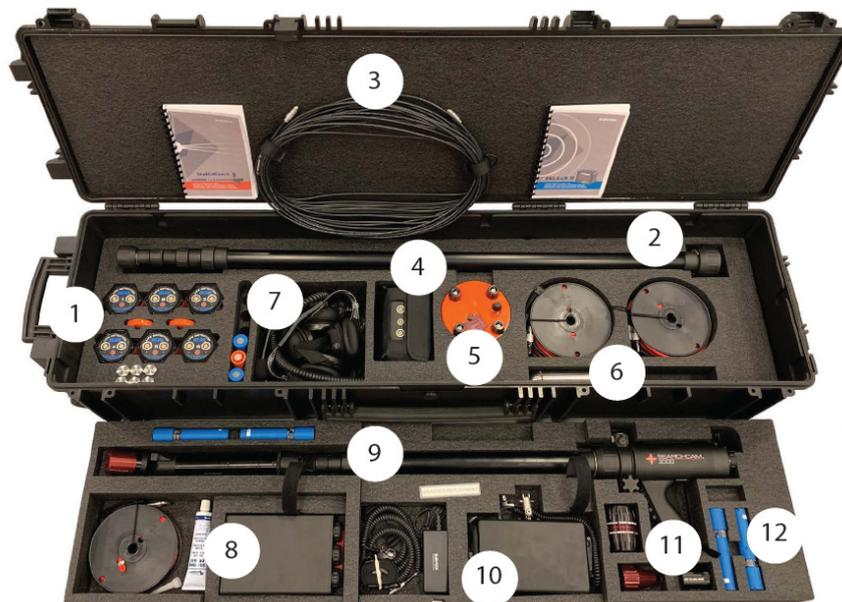
1. Seismic sensors
