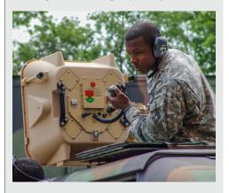
The LRAD 500X has been selected as the U.S. Navy and U.S. Army's AHD (acoustic hailing device) for small vessels and vehicles.
