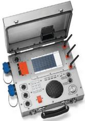
Fresh Air Base Station is positioned at the surface to act as the mission's command centre – tracking radiotelephones, monitoring node status, and issuing alerts as needed.
